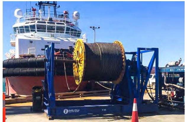
Spooling new 52mm Wire Rope on Forward Winch
